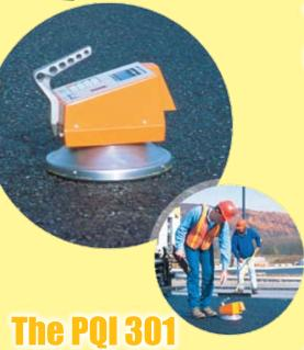
TransTech Model PQI 301 is a Pavement Quality Indicator designed and built to take quick, accurate measurements of hot mix asphalt density. Developed especially for today's perpetual pavement mixes, the PQI 301 enables the asphalt paving contractor, private testing organization or relevant jurisdiction to get on and off the mat fast, so as not to interfere with compaction.
