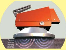
The PQI develops an electromagnetic field using a transmitter and receiver running at one megahertz, a frequency that falls between your AM and FM radio ranges. Transmission safety is not an issue – period! For more information, ask for a copy of TransTech's brochure entitled "Alternative to a Nuclear Gauge."
